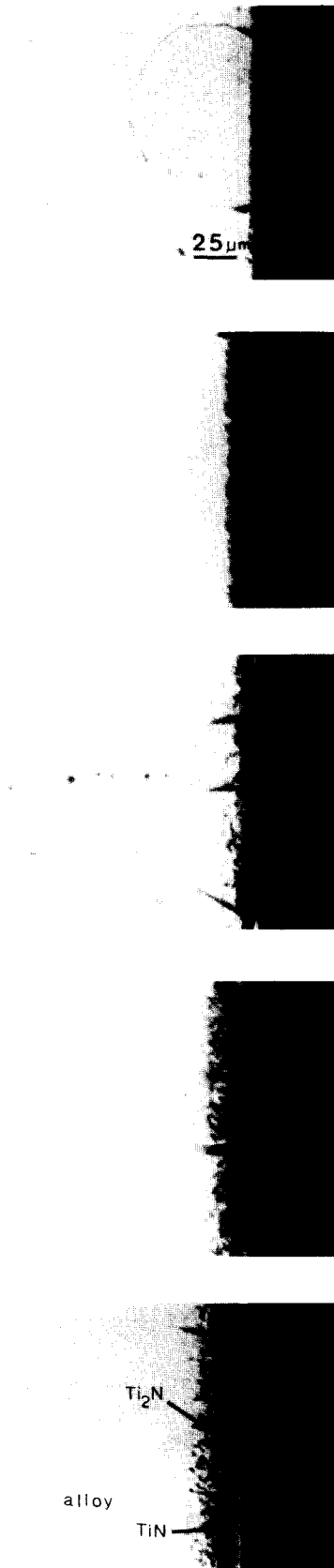
Fig. 3. Photomicrographs of the five nitrided plates after 180 min of nitridation: (a) 808 °C; (b) 857 °C; (c) 905 °C; (d) 957 °C; (e) 995 °C.
